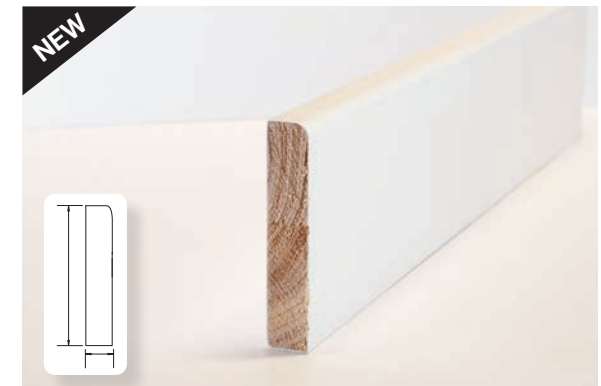
94 X 18 X 2185mm CONTEMPORARY ARCHITRAVE DELUXE PRIMED SOLID WOOD CORE FJ
