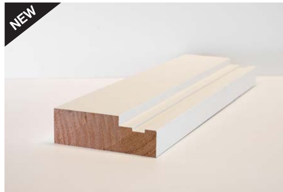
108/133 X 44 X 2100 mm DOOR FRAME REBATED FD30/EI30 (FIRE RATED) SOLID WOOD CORE FJ
