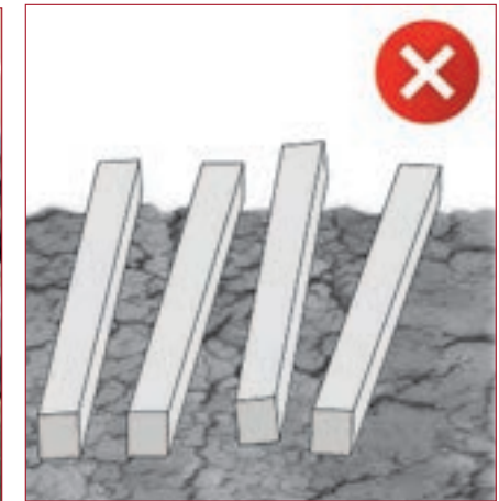
A structurally sound sub frame must be installed ensuring there is no movement prior to fixing boards to the joists. A 1.66% (1:60) fall to allow water to drain and a minimum 100mm free air space between the boards and the ground beneath to allow sufficient airflow to prevent the build up of moisture is essential.
